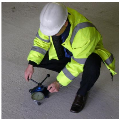
BS 8204: Part 3 The pull off should be >1.5 N/mm 2
